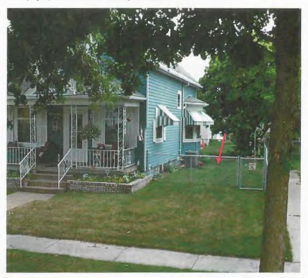
A six (6) ft. high fence would not comply with the side yard fence height requirements of the Zoning Code. Section 1145.17(g)(1) of the Sandusky Zoning Code permits a maximum height of 4.0 ft. for a side yard fence.
