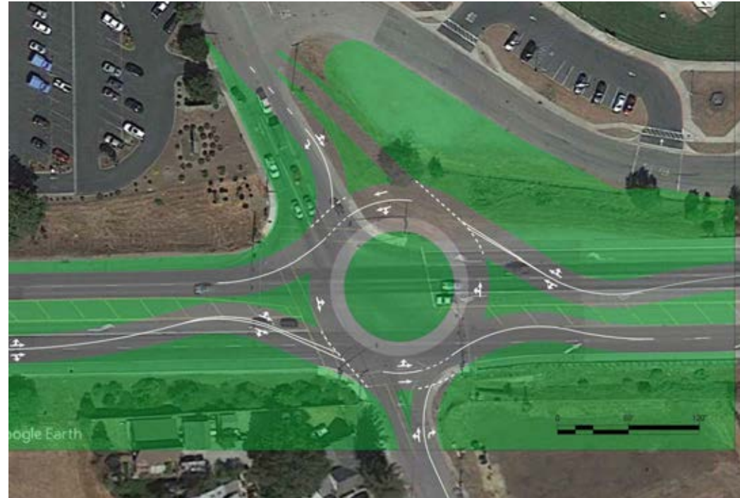
Proposed roundabout concept for The Alameda and SR-156 Developed During the June Charrette
