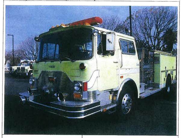
Mileage: Chassis: Body: Engine: Transmission: Pump Make/Model/Capacity: Water tank capacity: 124,411 miles Mack Weststates Mack 230 Allison Waterous, 1500 GPM 500 gallons
