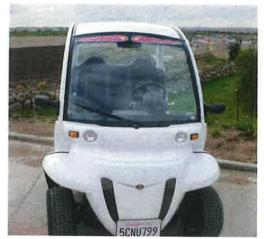
"The GEM (Global Electric Motorcar) is manufactured in Fargo, North Dakota and sold by Chrysler dealers. It is a street legal electric vehicle with 3-point seat belts, safety glass windshield, head and tail lights, turn signals, four wheel hydraulic brakes, independent front suspension, 72-volt motor, six 12-volt batteries, approximate driving range is 30 miles on one charge."
