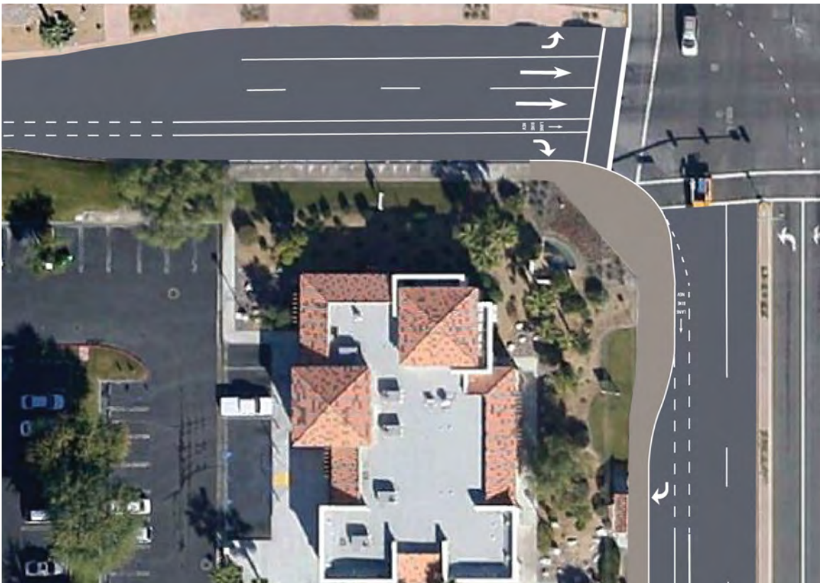
Figure 28: Typical Right-turn Departure NEV/Bike Lane
