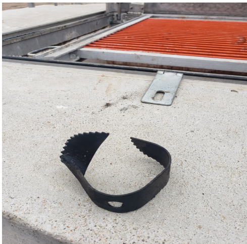
this picture shows the sewer snake cutter that damaged pump #2
