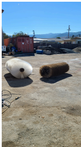
Street Sweeper worn out main broom compared to the new broom.
