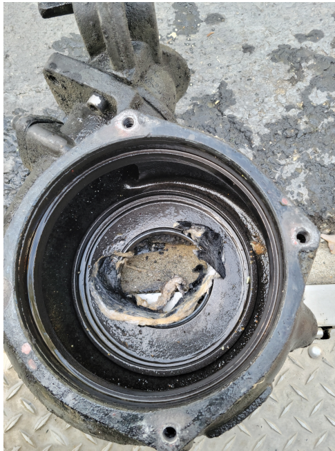
Ahwahnee Sewer lift station pump clogged up
