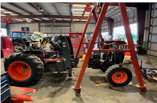
Public Works backhoe during the engine replacement process very extensive job
