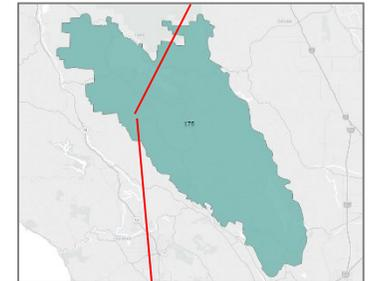
Decision is made on a transmission line level that intersects within a weather footprint
