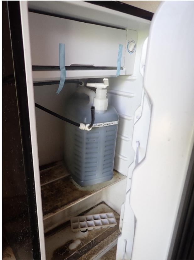
*Photo 17 : Refrigerator containing composite sample container.*
