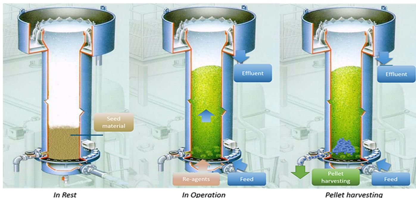
**Figure 7 Pellet Reactor Column Schematic (Procorp® Crystalactor)**
