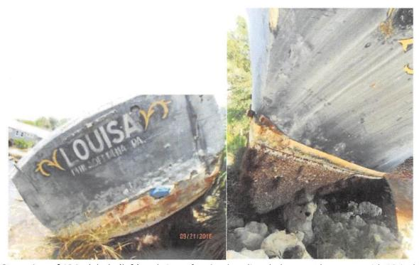
Stern view of 12 inch hole (left) and view of rocky shoreline, below port bow area with 10-inch hole created by protruding rock (right).
