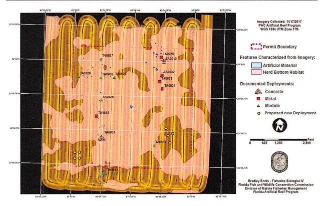
Module spacing/layout: At least eight (8) pre-fabricated modules must be deployed at each of the 8 reef deployment sites mentioned above, creating a reef patch. Two grouping of four modules by each side of the barge. Pre-fabricated reef modules patches will be placed no more than 30 ft apart from each other.
