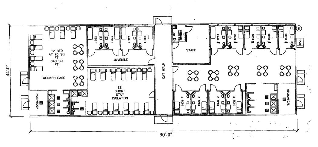
Floor plan illustrates a building size of  $44' \times 127'$ . Some rooms may be repositioned, eliminated and/or overall floor plan revised to result in a  $44' \times 90'$  building dimension. The Staff Area, a mechanical room and a single cell are acceptable removals.
