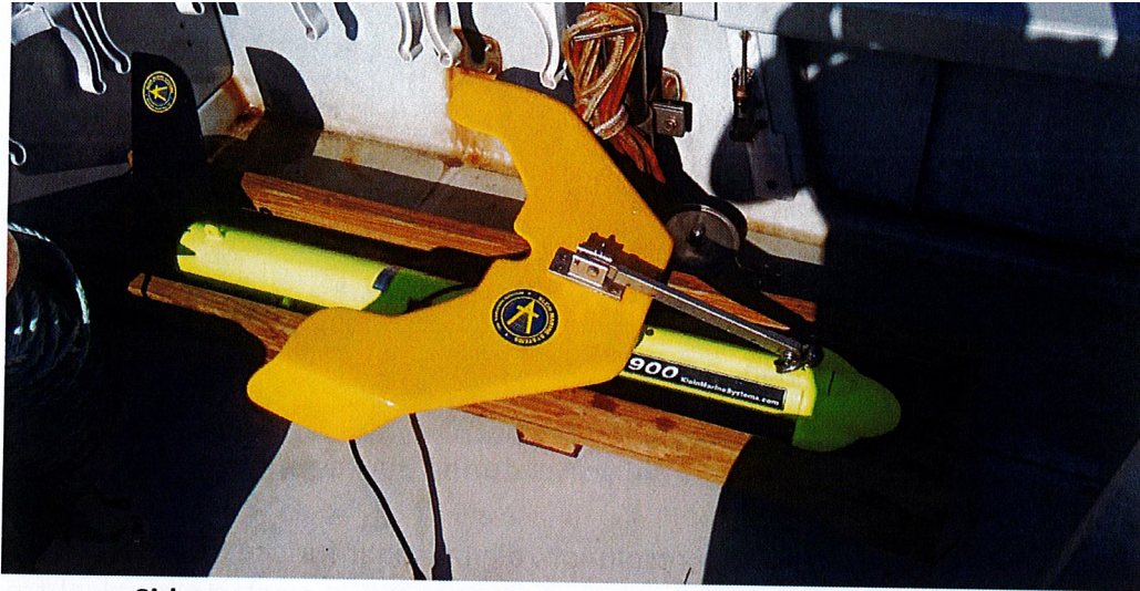
Side scan system at FWC vessel during Buckeye Reef survey.
