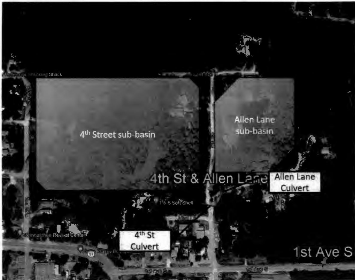
Figure 6-3: Alternative Culvert Layout
