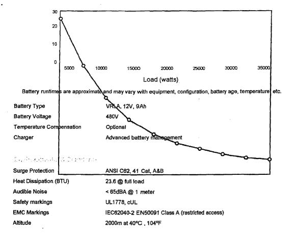
1. Due to continuing improvements, specifications are subject to change without notice. 3. At full load without battery discharge. 4. Output transformers are required if the desired output voltage is not the same as the input voltage. 5. 600V applications require an output transformer.
