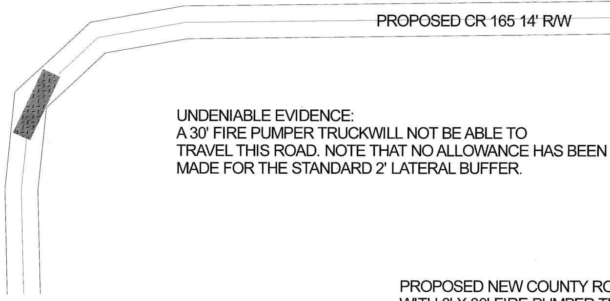
PROPOSED NEW COUNTY ROAD 165 WITH 8' X 30' FIRE PUMPER TRUCK OR SIMILAR VEHICLE. SCALE: 1" = 20'
