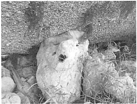
Photo 7. Rock creating 10-inch hole at port bow.
