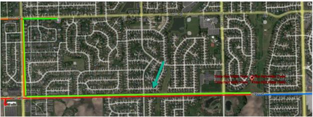
Green represents new Conduit and fiber for use by Tinley Park to be installed by County. (Fiber will be pulled through existing Tinley Park conduit at the water tower location.)
