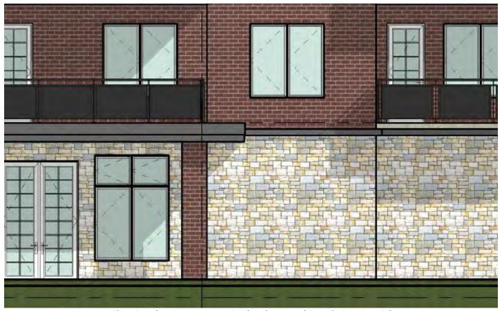
Elevation Showing Precast Stained and Stamped Foundation Material
