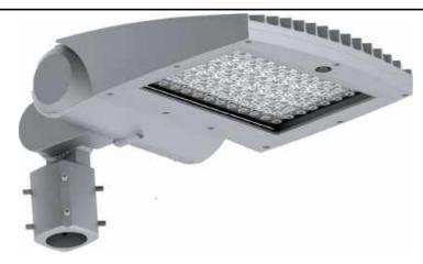
An adjustable knuckle slip fits over a 2-3/8" Tenon, and allows for up to 90 degrees of vertical adjustment in 10 degree increments from horizontal, as well as full side to side adjustment with the knuckle mount.
