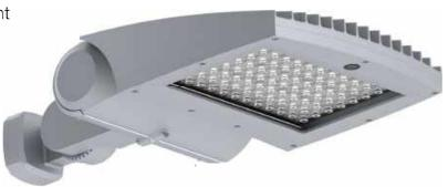
An adjustable knuckle that threads onto a ¾" NPT, and allows for up to 90 degrees of vertical adjustment in 10 degree increments from horizontal.
