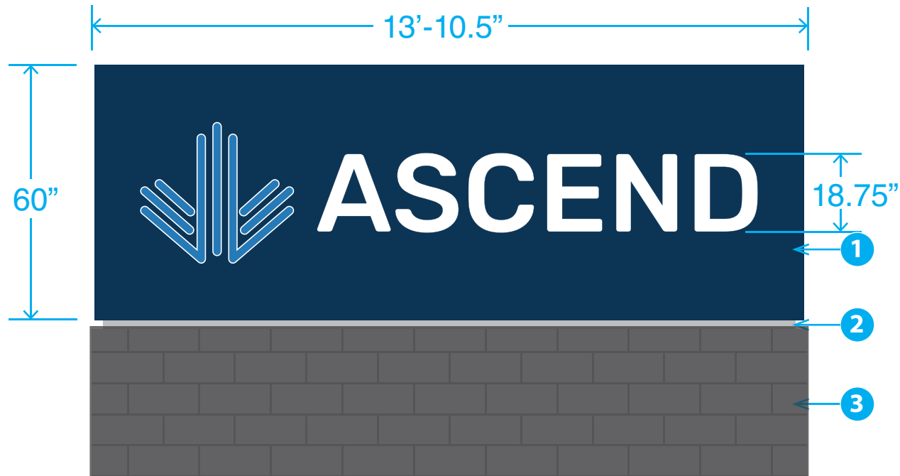
D 1 SIGN DETAIL - Dimensions SCALE: 3/8" = 1'
