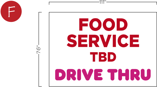
NORTH ELEVATION ILLUMINATED CHANNEL LETTER WITH WHITE BACKER 58.5 SQ. FT. 1/4" SCALE
