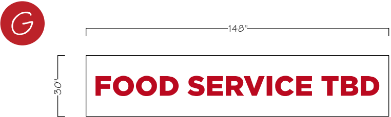
WEST ELEVATION ILLUMINATED CHANNEL LETTER WITH WHITE BACKER 31 SQ. FT. 1/4" SCALE
