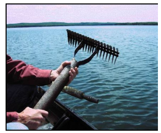
Barr's subcontractor, Endangered Resource Services LLC, used a rake (pictured above) to collect plants for the surveys. Rake fullness is a measure of plant density. Photo Credit: Endangered Resource Services LLC
