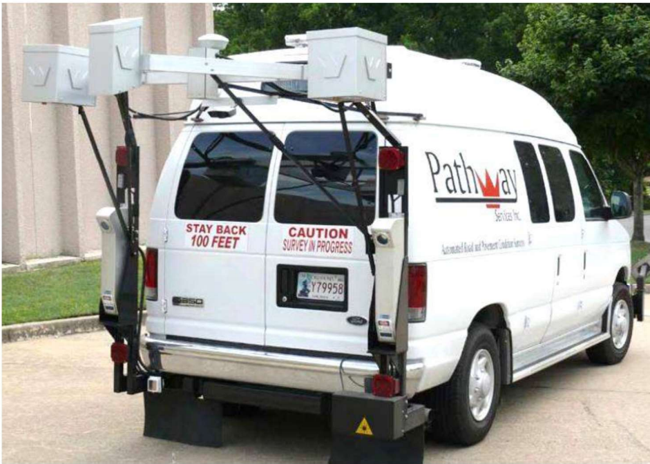
Figure 2: A “Pathrunner” Automated Data Collection Vehicle (Pathways) This is one of the van’s that a previous data collection vendor used to collect pavement condition in Iowa from 2013-2017.
