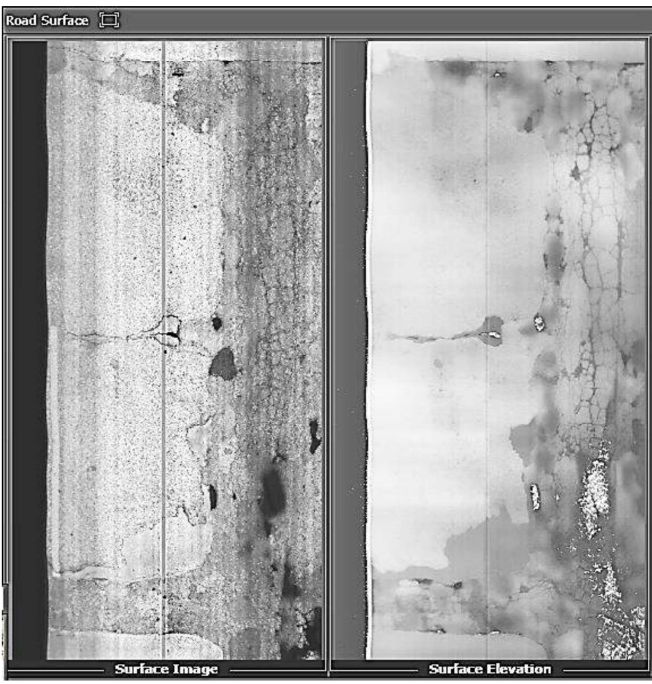
Figure 22: Roadway Imagery of a “Very Poor” PCC Pavement This image is from the section of Fletcher shown in Figure 21. These were captured by the data collection vehicle’s downward facing camera (left) and LIDAR array (right). These are one of the key resources used in evaluating pavement condition.
