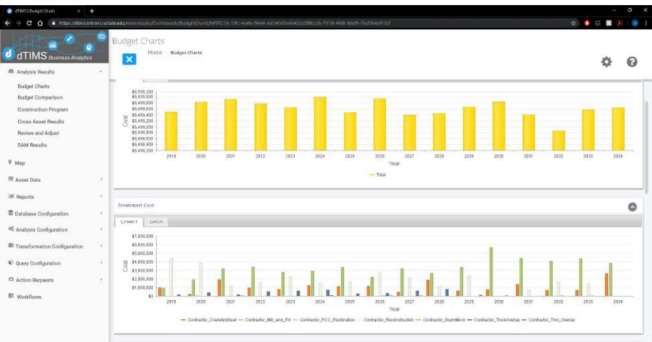
Figure 23: dTIMS BA Interface The dTIMS BA software is accessed through normal computer browsers and operates over cloud-based technology. Calculations are performed on remote servers, meaning any computer can use it, regardless of hardware capabilities!
