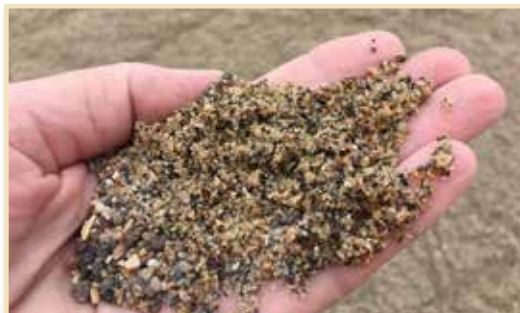
Concrete sand is added to rain gardens to enhance percolation.
