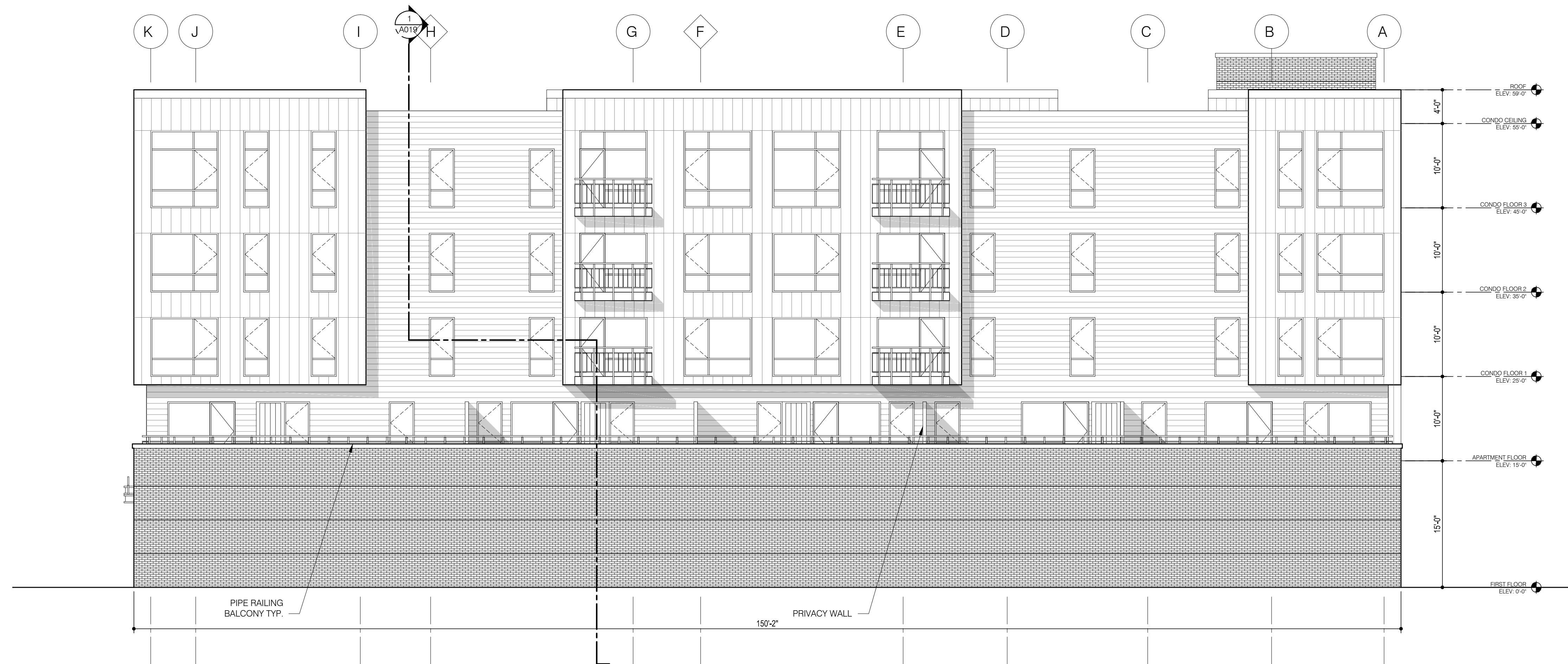
1 A018 East Elevation 1/8" = 1'-0"
