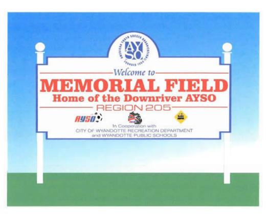
4' by 8' MDO plywood sign, one sided installed on 4" by 4" post with pvc covers and finial tops cemented in at base
