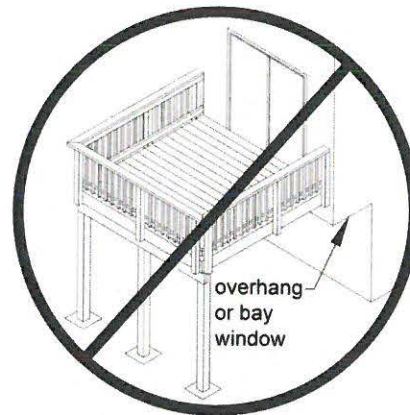
Figure 18. No Attachment to House Overhang with Ledger.
